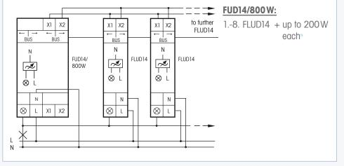
Capacity increase for additional lamps (춘추) in dimmer switch operating modes AUTO, LC4, LC5 and LC6. For operating modes EC1, 2 and LC1, 2, 3, see next page.
