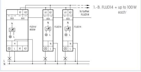
$^{\circ}$  Ventilation clearance of  $\frac{1}{2}$  module to adjacent devices must be maintained.
