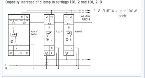
Capacity increase with additional lamps in settings EC1, 2 and LC1, 2, 3.
