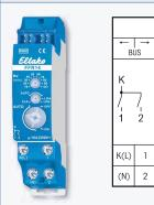
2-channel mains disconnection relay, 1+1 NO contacts potential free 16A/250V AC, incandescent lamps 2000 watts. Bidirectional. Only 0.1 watt standby loss.
