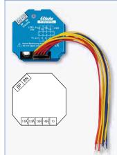
Bus pushbutton coupler FTS61BTKL for 4 conventional pushbuttons with integrated 24V LEDs for connection to FTS14TG pushbutton gateways by 2-wire pushbutton bus. Only 0.2 watt standby loss.
