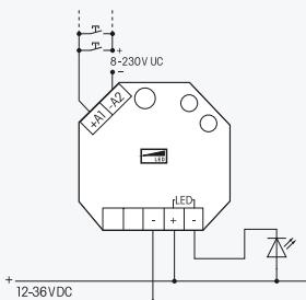
**PWM LED dimmer switch for LEDs 12-36V DC, up to 4A. Only 0.2-0.4 watt standby loss. With adjustable minimum brightness and dimming speed. With switching operation for children's rooms and snooze function. Also with light scene control by PC or wireless pushbuttons. Encrypted wireless, bidirectional wireless and repeater function are switchable.**
