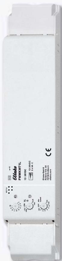
**PWM dimmer switch with 2 channels for LED 12-36V DC, each up to 4A. Input: two terminals each for + and -. Output: one terminal for +, two terminal each for channel 1 (warm white) and channel 2 (cold white). Adjustable minimum brightness and dimming speed. With snooze function and light alarm circuit. Additionally with light scene control via PC or with wireless pushbuttons. Activation for encrypted wireless, bidirectional wireless and repeater function. Standby loss only 0.3-0.5 watt.**
