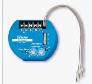
Powerline Venetian blind actuator for 1 motor. 53x43mm, 25mm deep for mounting in 58mm switch boxes. 1+1 NO contact for motors up to 3A. 2 sensor inputs with internal low voltage. Standby loss only 0,5 watt. To control and switch at the same place.
