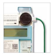
AIR IR scanner for energy meters
