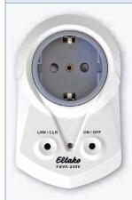
1 NO contact not potential free 10 A/250 V AC, incandescent lamps up to 2000 watts, ESL and LED up to 400 W. With integrated current measurement up to 10 A. Encrypted wireless, bidirectional wireless and repeater function are switchable. Only 0.8 watt standby loss.
