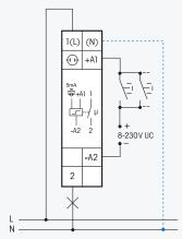
**or** control voltage 230 V with glow lamp current up to 5 mA
