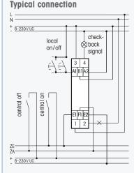
By using a bistable relay coil power loss and heating is avoided even in the on mode. The switched consumer may not be connected to the mains before the short automatic
