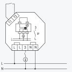
The power supply of an extractor hood is connected by a window contact (NO if window open) so it can be switched on only if the window is open.
