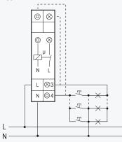
3-wire circuit, resettable
