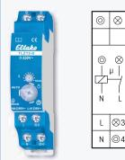
1 NO contact not potential free 16A/250V AC. Incandescent lamps up to 2000 W, energy saving lamps ESL and LED lamps up to 100 W, without switch-off early warning. Standby loss 0.7 watt only.
