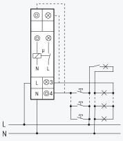
4-wire circuit with attic lighting, resettable
