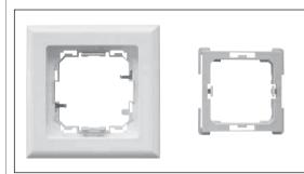
2. Remove the mounting frame from the frame. To unlock, press the tab on the top and bottom to the outside.
