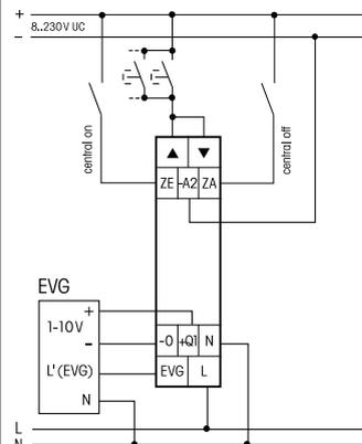
At more than 2 devices side by side, an half pitch must stay free for ventilation. For the control from several LED drivers with 1-10V passive interface, an additional voltage source is necessary, this can be the power supply unit SNT12-230V/12V DC-0.5A or SNT61-230V/12V DC-0.5A, in both cases a 1kOhm resistor is necessary.
