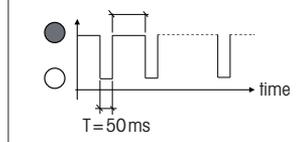
Energy meter correctly connected, with power consumption
