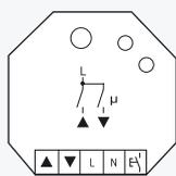
**1+1 NO contact not potential free 4A/250V AC, for roller blinds and shading systems. Encrypted wireless, bidirectional wireless and repeater function are switchable. Only 0.8 watt standby loss.**
