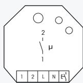
**1 NO contact potential free 10A/250V AC, incandescent lamps up to 2000 watts, off delay with switch-off early warning and switchable push-button permanent light. Encrypted wireless, bidirectional wireless and repeater function are switchable. Only 0.8 watt standby loss.**
