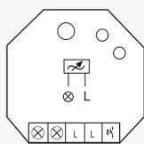
**Without N connection, power MOSFET up to 300W. Only 0.7 watt standby loss. With adjustable minimum brightness and dimming speed. With switching operation for children's rooms and snooze function. Light scenes can be taught-in. Encrypted wireless, bidirectional wireless and repeater function are switchable.**
