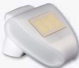
The MS multi sensor sends the current weather details, including brightness (from three points of the compass), wind, rain and frost, to the weather data transmitter module FWS61 connected in series once per second. A standard telephone wire is sufficient as connecting lead: J-Y(ST)Y 2x2x 0,8 or equivalent. 100m line length is permitted.
