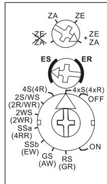
With the upper rotary switch this impulse switch with integrated relay function can be partly or completely excluded from central control:
