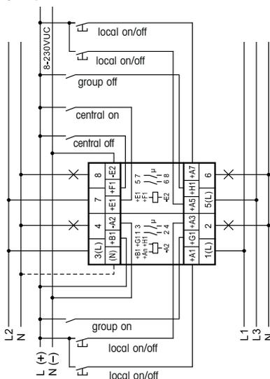
If N is connected the zero passage switching is active at the contacts 1-2, 3-4 and 5-6.
