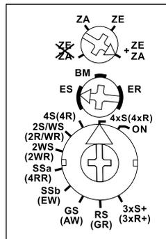
**With the upper rotary switch** this impulse switch with integrated relay function can be partly or completely excluded from central control:
