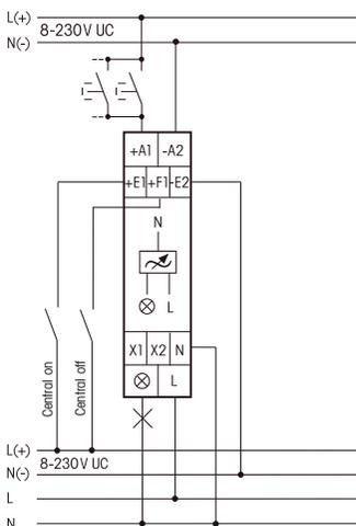
**Function 'DSD'** = Same as universal dimmer switch EUD but also comprising activation via two direction switches on the universal voltage control inputs 8..230V UC.
