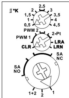
First teach in the sensors **using the rotary switches**. In normal mode, set the operating mode using the middle rotary switch.
