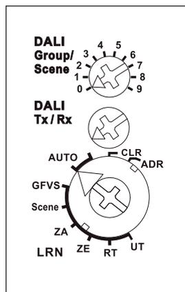
**Operation:** After switching on the power supply, the complete DALI bus is scanned after the RS485 bus scan of the FAM14. The green LED of the FDG14 then flickers for several seconds. All existing DALI devices are detected together with their short addresses and the minimum brightness (MIN LEVEL), dimming speed (FADE RATE) and group assignment saved in the DALI device are read out. The least possible minimum brightness is determined from this data
