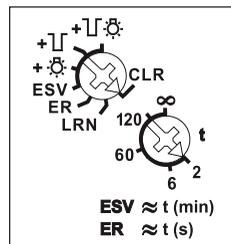
**With the top rotary switch** in the setting LRN up to 35 wireless pushbuttons can be assigned, of which one or more central control pushbuttons. In addition wireless window/door contacts with the function N/O contact or N/C contact while the window is open. The required function of the impulse switch with integrated relay function can then be selected:
