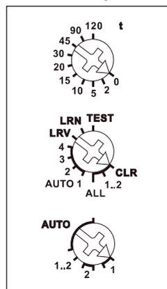
**Use the rotary switches** to teach-in the pushbuttons and test the 2 channels as required. For normal mode, the middle and lower rotary switches are then set to AUTO. With the upper rotary switch the EW time (0-120 seconds) is directly set for relays or the RV time (0-120 minutes) for impulse switches for all channels if necessary.
