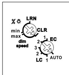
The minimum brightness (fully dimmed) or the dimming speed is adjustable **with the upper %/dimming speed rotary switch.**
