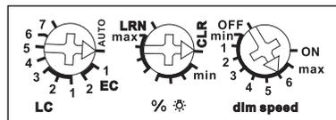
**The left rotary switch** on the side is required first for teach-in. In operation, the release delay is set by FBH or the staircase light pushbutton in minutes.
