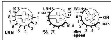
The minimum brightness (fully dimmed) is adjustable with the % rotary switch on the side. In the setting LRN up to 30 wireless pushbuttons can be assigned, of which one or more central control pushbuttons.
