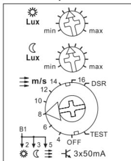
**Lux ☀️** = This rotary switch is used to set the brightness 1 klux-60klux at which the **Sun signal** is immediately triggered as a 2-second pulse on output 2. The LED behind the rotary switch indicates when the brightness value is exceeded.
