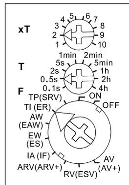
The LED below the big rotary switch indicates the contact position while time-out is in progress. It blinks while the relay contact 15-18 is open (15-16 closed), and is continuously ON as long as the relay contact 15-18 is closed (15-16 open).
