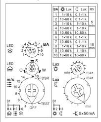
BA = Setting of the operation modes 1 to 10 from the adjacent chart. 2 delay times RD - for wind and twilight - each in connection with 5 brightness ranges for light and twilight. The LED behind the rotary switch indicates Frost at an outdoor temperature below 2°C, at this point output 6 is closed. This output opens again as soon as the temperature is above 3°C for 5 minutes.
